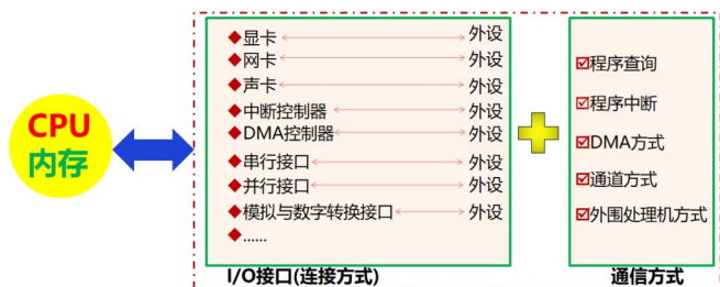
Fig. 1 Basic composition of I/O system
